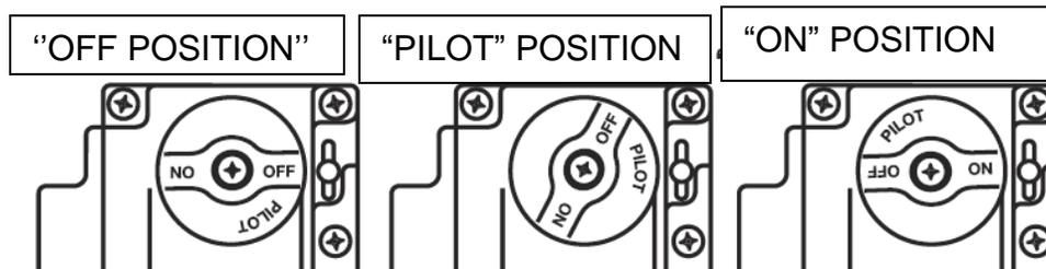
3. While pressing the knob down, use a lit match to ignite the pilot. Continue to press the knob down for about 30 seconds. If the pilot does not stay lit when the knob is released, repeat the lighting procedure and keep the knob down longer. Adjustment of pilot flame may be necessary.
