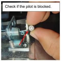
If confirmed that the pilot nozzle is not blocked, and still unable to ignite the pilot, , the gas valve needs to be replaced.
