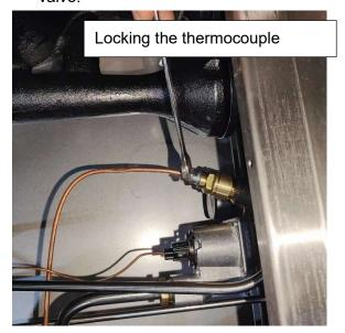
• If the trouble still occurs, you should remove the thermocouple connector from the gas valve end, and clean the end of the thermocouple with a cloth and reinstall it for locking.
